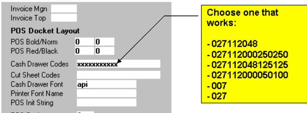
The image shows a screenshot of the Peach Business Software settings window, specifically the 'POS Docket Layout' section. The 'Cash Drawer Codes' field contains 'xxxxxxxxxx'. An arrow points from this field to a yellow box on the right containing a list of codes to be tested. The yellow box contains the following text:
