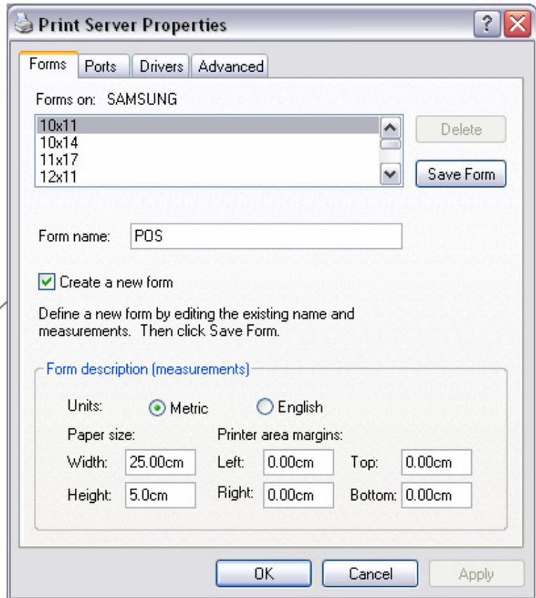
Click on the 'Create New Form' option; then type in the form name: 'POS' And fill in the paper size as shown at the bottom.
